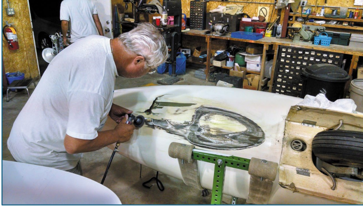
Photo #83: Emergency repair from gear-up landing. Fuselage upside down: landing gear and gear doors to the right; teardrop-shaped damaged area in middle.
