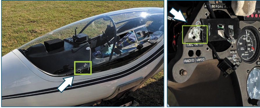
Photos #86 & 87: Bullet passed through trailer skin (layer 1); upper/lower wing surfaces (layers 2 & 3); punctured canopy (layer 4) and instrument pod (layer 5)—note arrow; then exited instrument panel (layer 6)—note arrow, with missing power switch and fuses; before breaking larger hole in canopy, (layer 7)—see following photo.
