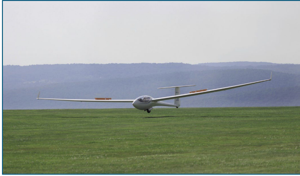
Photo #63: ...and landing (note extended dive brakes). (photos at Elmira, New York, 2015, by Guerry Howard)
