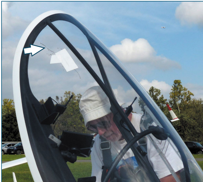
Photo #88: Canopy damage, with white speed tape over the hole and cracks radiating from it. (photo by Nirmal Mathrani)
