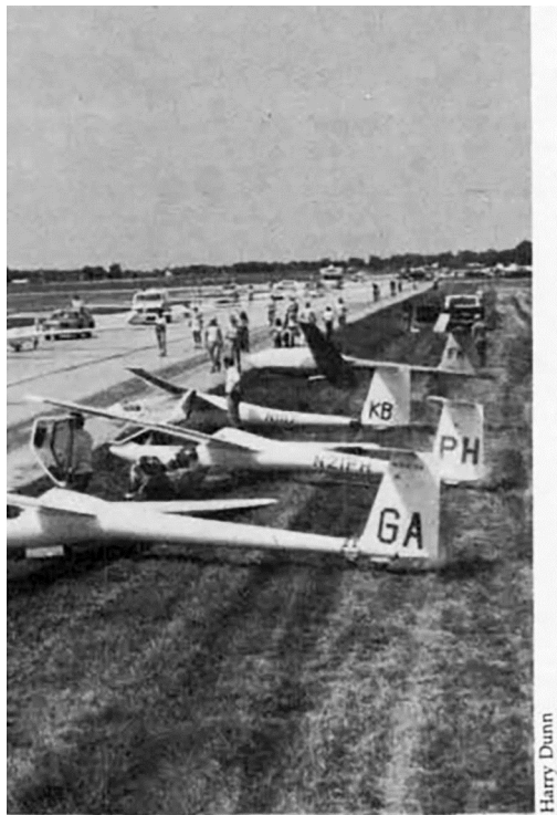
Photo #46: Springfield launch grid: crews pull each glider down the taxiway to its grid number, then push it into the grass to leave room. The last step is moving the gliders to the taxiway in single file. (photo by Harry Dunn, from Soaring magazine, October 1980, used with permission).
