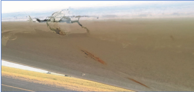
Photo #84: Leading edge and lower surface of wing after striking landing light.
